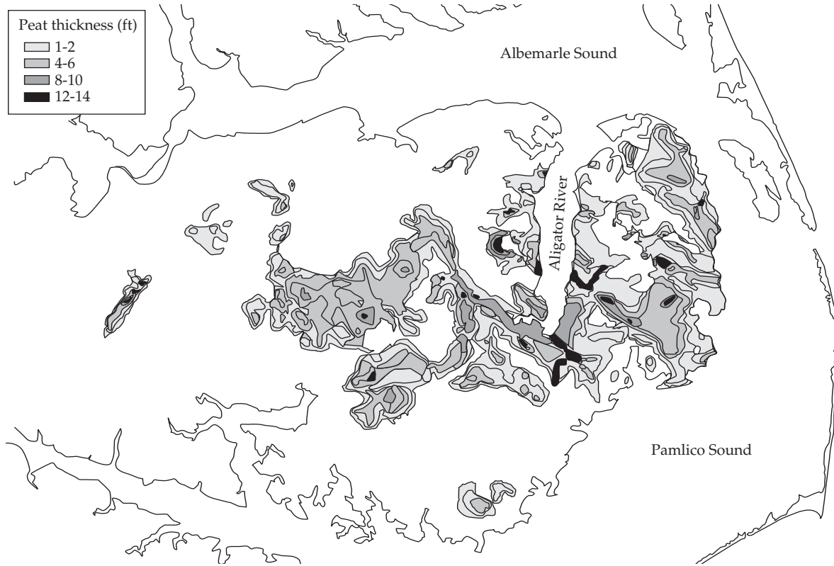
Figure B Thick peat deposits on the Albemarle Peninsula are vulnerable to salt water intrusion due to sea level rise. Numerous ditches throughout the region can bring rising sea water further inland, where the thickest peat deposits can be destroyed. (Modified from Poulter 2005.)
