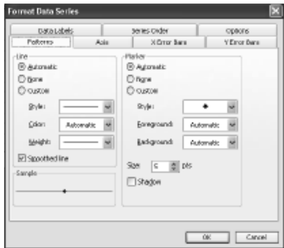
Figure A2.10 Patterns tab inside Format Data Series dialog box, opened by double-clicking a data series (line or symbol) on a line graph
