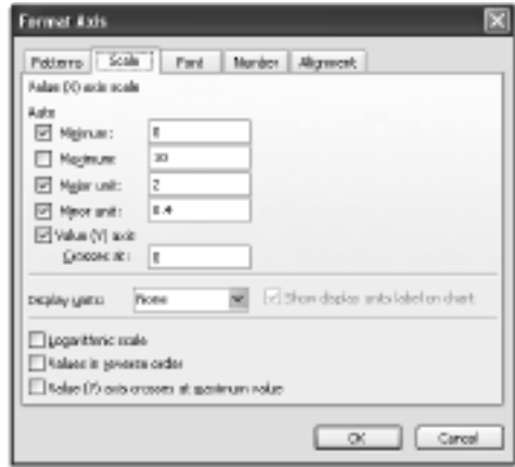
Figure A2.11 Scale tab inside Format Axis dialog box, opened by double-clicking any number on either the y -axis or the x -axis
